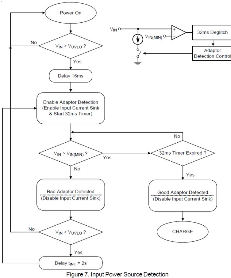
Figure 7. Input Power Source Detection
