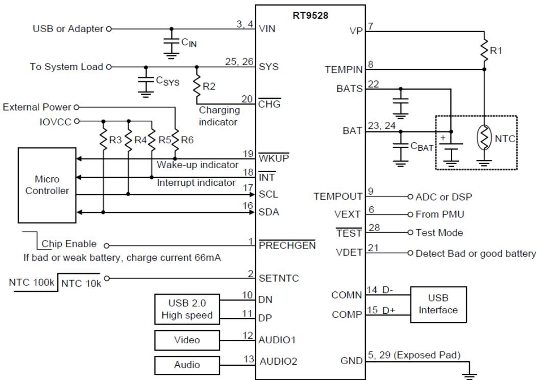
Figure 10. RT9528 application circuit.
