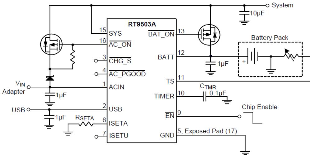
Figure 7. Typical application circuit of the RT9503A.
