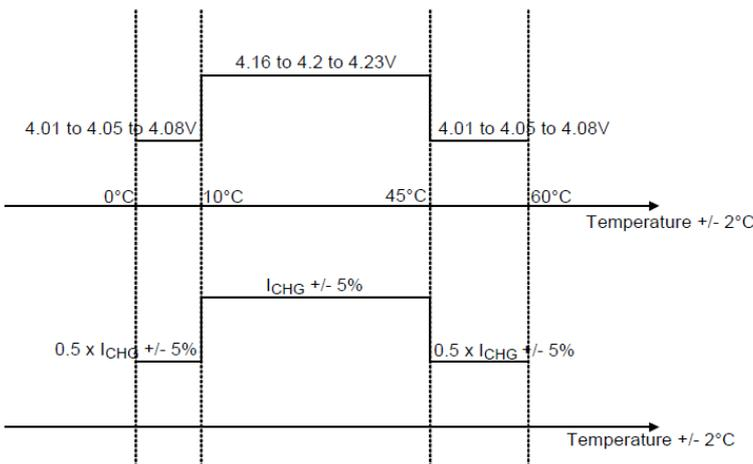
Figure 8. Battery charger solution for JEITA compliance.
